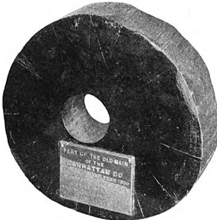
Section of wooden water pipe laid under the streets of New York City by the Manhattan Company in 1799, for the purpose of supplying "pure and wholesome water to the citizens of New York," as provided by its charter. Sections of this pipe were dug up over 100 years later in a fine state of preservation
