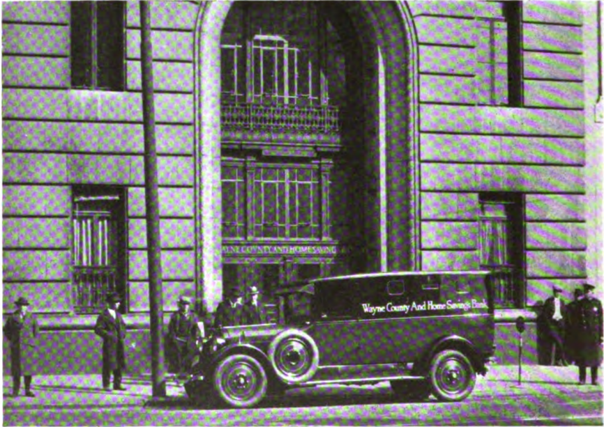
Armored car built for the Wayne County and Home Savings Bank of Detroit by the Cadillac Motor Car Company
