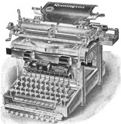
Remington Typewriter with Wahl Attachment and Two Totalizers.
