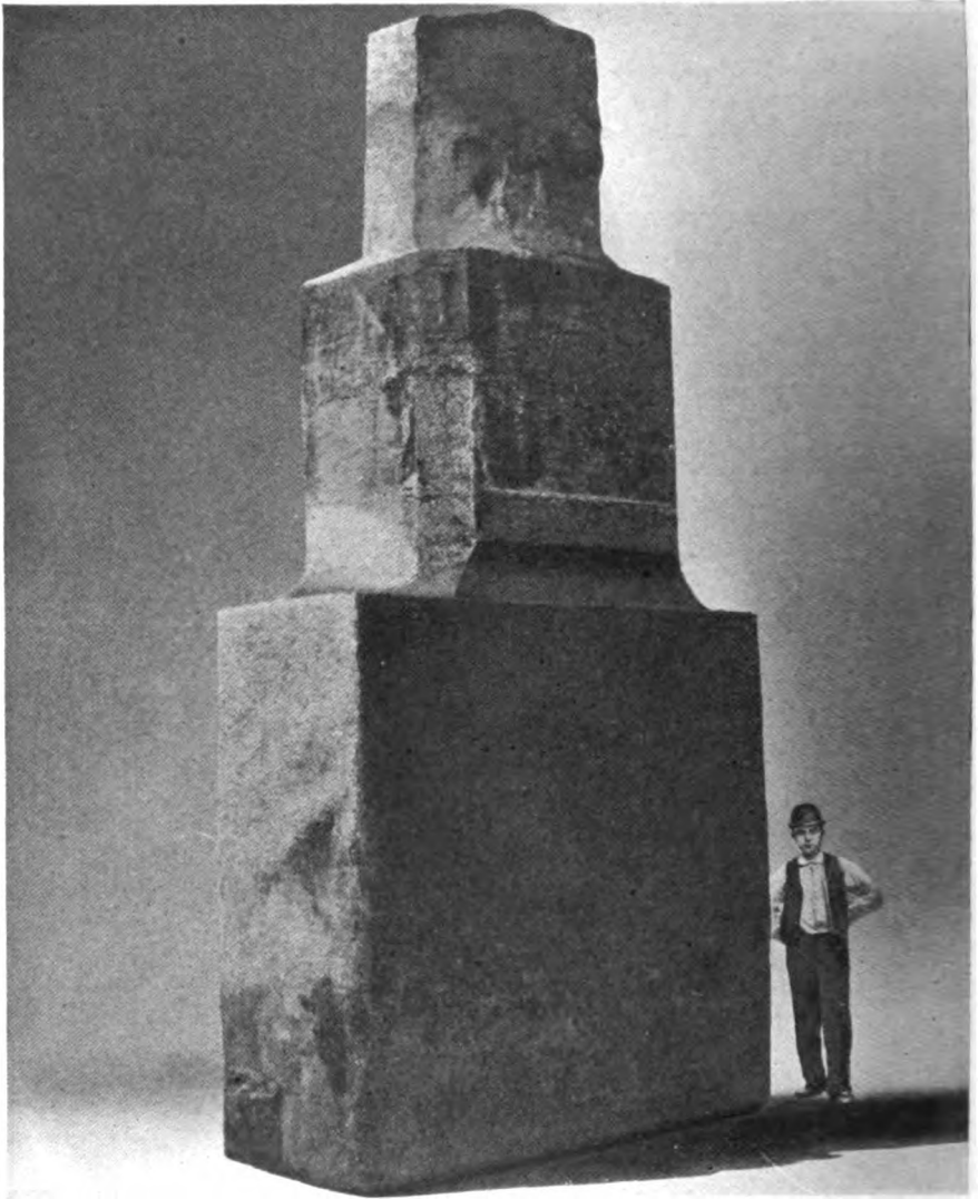
AN INGOT FROM WHICH ARMOR PLATE IS FORGED. WEIGHT, 273,500 LBS.
