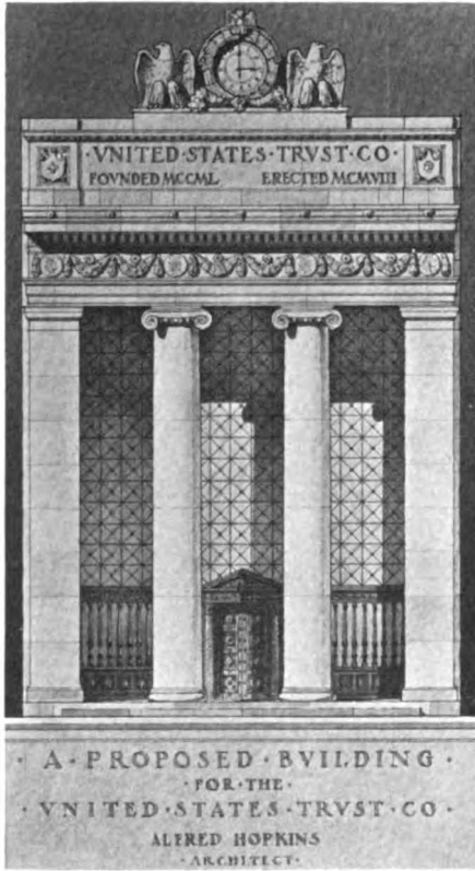
Design for a bank on an interior lot, showing a method which obtains the maximum of light behind the columns. The lot is 40 feet in width, perhaps a minimum for this type of design
