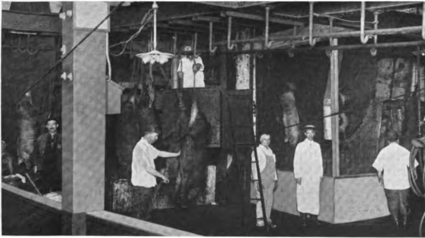
Hog Killing, View Showing Pig Wheels in Action, Armour and Company, Chicago
